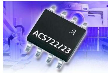
Fig.4. Circuito integrado ACS723 de Allegro Microsystems.
