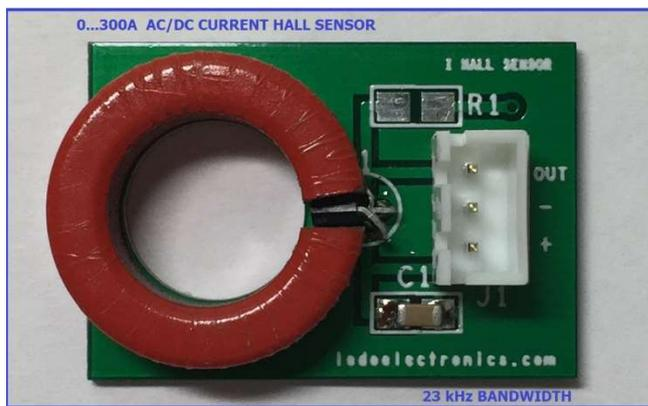
Fig.9. Linear Current Hall Sensor.
