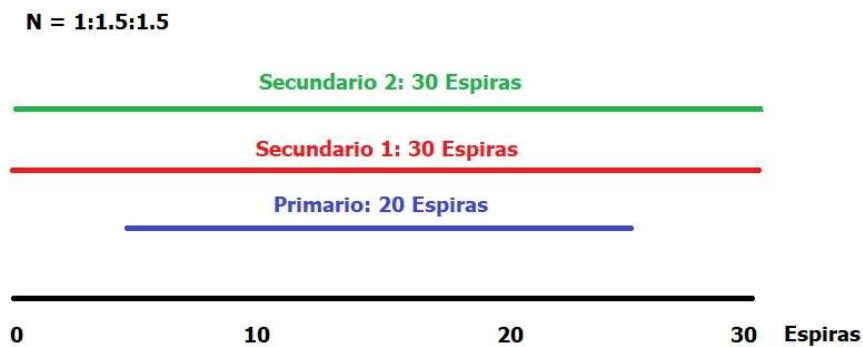
Fig.4. Three-wire winding of a pulse transformer
