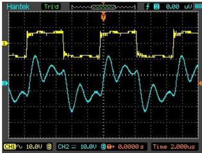
Fig.2. Passing a 106 kHz pulse through the Murata 1002C transformer to a 50A MOSFET Gate.
