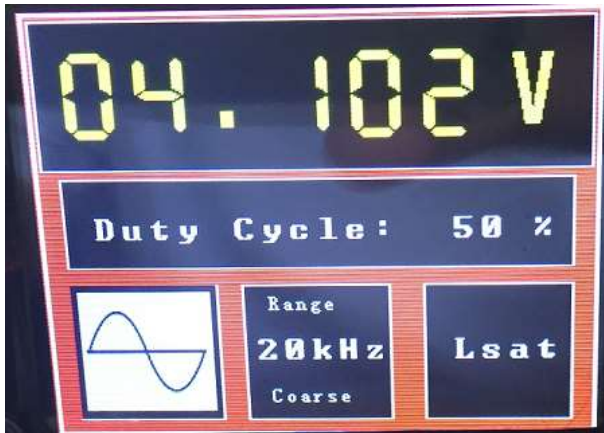
Fig.16. Automatic representation on the screen of the power supply voltage.
