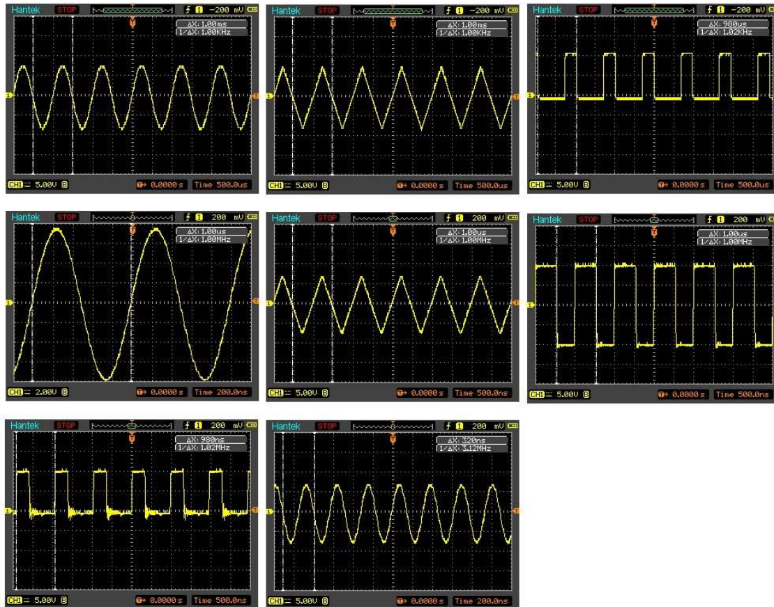
Fig.2. Different waves generated by the equipment.
