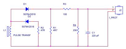
Intended for the measurement of high frequency current in power converters of all kinds. The conductor whose current is to be measured must be introduced through the toroidal core.
